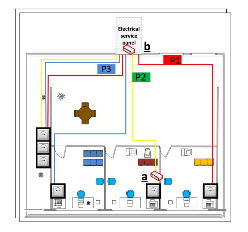
According to their testing, binary data can be extracted through the power lines at bit rates of 1000 bits per second for the first attack and 10 bits per second for the second.
